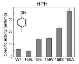
FIGURE 4: Specific activities of the BstHYD variants generated by saturation mutagenesis at position 159. In a mutant library, the enzymes with high activity for HPH were selected, and their specific activities for various substrates were determined.
